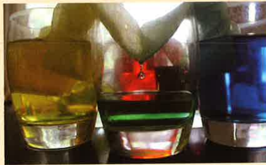
▲ Figure 4 The ability of adhesive forces to result in the movement of water is demonstrated in this image. A folded paper towel with one end immersed in water will transport water into an empty container by capillary action
