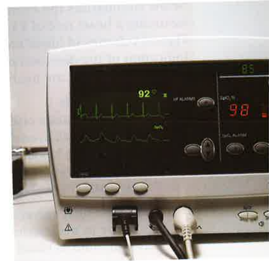
▲ Figure 13 Heart monitor displaying the heart rate, the electrical activity of the heart and the percentage saturation with oxygen of the blood
