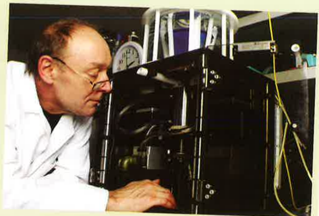
▲ Figure 10 The Dynamic Gastric Model with its inventor, Richard Faulks, adjusting the antrum mechanism
