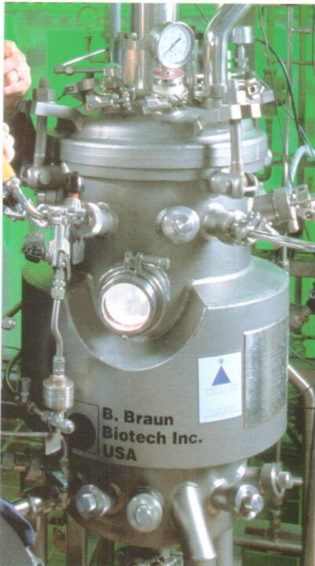
This is a bioreactor and is used to grow bacteria which have recombinant DNA.
