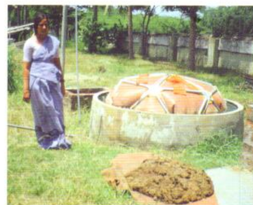
Using a small-scale biogas digester such as this one in India, farmers can trap methane instead of letting it escape from rotting manure into the environment. Methane from farms is a significant greenhouse gas.
