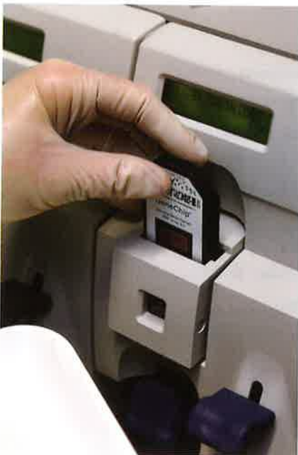
▲ Figure 7 A DNA microarray cartridge being loaded into a machine that will be used to analyse the results from this test
