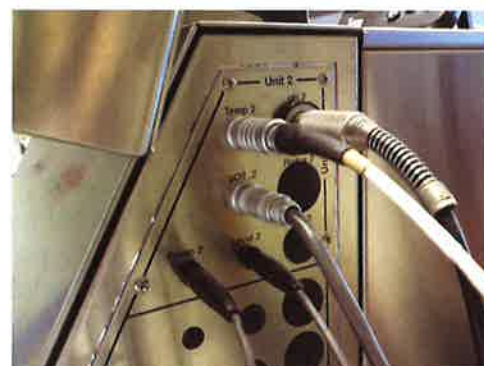
▲ Figure 5 A system of probes is connected to the fermenter to monitor conditions within the vessel
